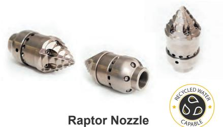
The Raptor Nozzle is a powerful nozzle capable of removing heavy obstructions caused by roots, grease, or any other solid organic material quickly. Its tempered stainless steel drill head is turbine-driven and spins in the range of 6,000 rpm and 12,000 rpm. The Raptor Nozzle succeeds where standard hydromechanic tools
