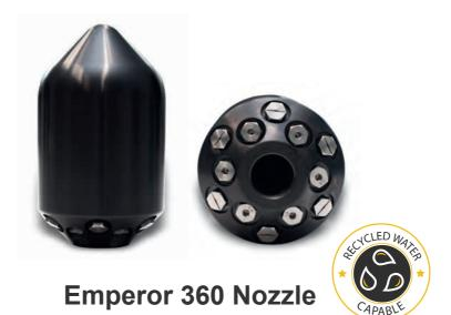
This high-performance nozzle is perfect for removing hard grease and scale that may be encrusted on the circumference of the pipe. The fan jets clean the pipe interior streak free  $360^{\circ}$ , while the propulsion nozzle inserts provide superior movement of obstructions such as encrusted grease, scale etc. to the manhole. The Emperor 360 nozzle is an indispensable, hydromechanical tool prior to video inspection.
